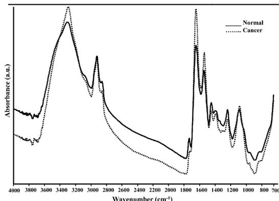
**Figure 1:** Overlaid Infrared Spectra of Normal and Malignant Lung Tissue in the Region 4000-700  $\text{cm}^{-1}$
